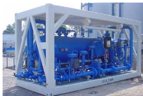
Three Phase Test Separator
