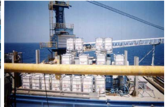
Package Allows Safe and Secure Storage of DE Material in Staged Intermediate Bulk Carriers
