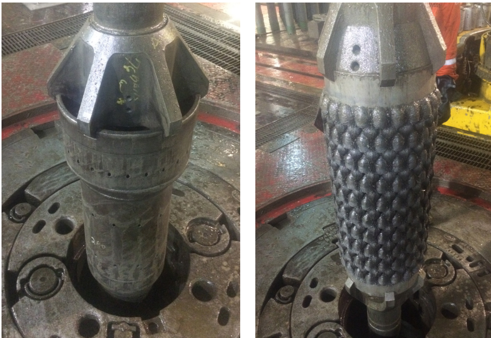
Effective junk basket and riser magnet clean up using TADS-SF displacement system.
