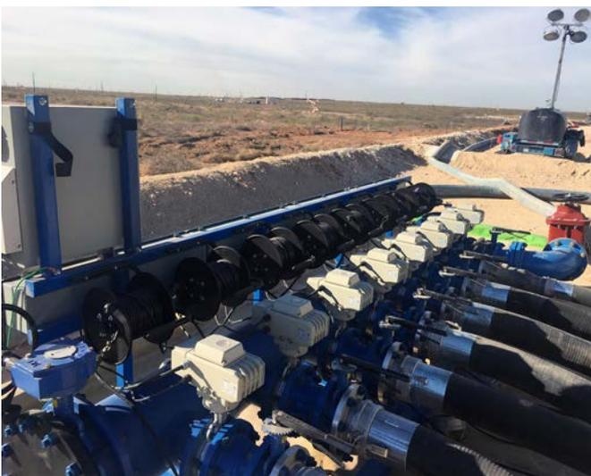
**Figure 3.** The TETRA automated distribution manifold helps manage frac water buffer volumes safely and efficiently. The manifold provides real time computer-controlled management of tank level to ensure supply and prevent tank overflows.
