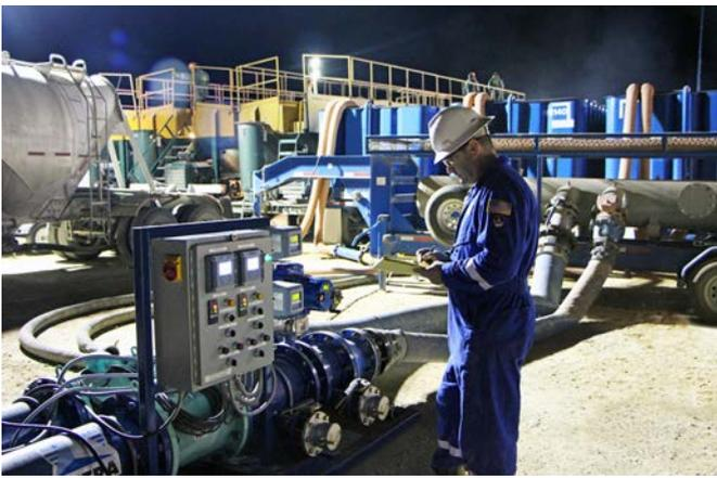
**Figure 2.** The TETRA frac water blending system includes an automated blending controller, coupled with a patented, on-the-fly blending manifold. The combination provides accurate parameter-based blending and consistent blend quality, whether directly filling frac tanks or transferring to another location.
