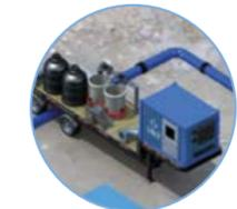
**Automated Treatment** – The TETRA advanced treatment system provides continuous and accurate chemical dosage volume. This ensures that your produced water is optimized to your exact specification.
